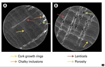
**Figure 3: Segmentation diagram of lenticels on 3D tomographic images based on segmented stoppers.**
