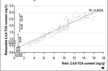
TCA (ng/g) or releasable TCA (ng/L) in the closure. The total TCA content (ng/g) present in the closure is measured after grinding, extraction with an organic solvent and analysis by isotope dilution using gas chromatography (GC) coupled with mass spectrometry (MS) in fragmentometric mode (SIM).
